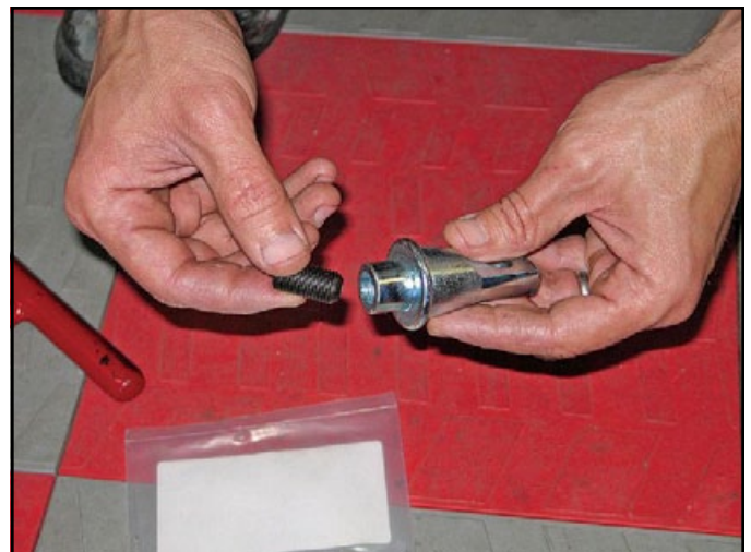
Begin assembly of the coilover shocks by threading one of the 1/2-inch set screws into one of the crossbar halves. Then place an aluminum crush washer over the remaining part of the set-screw.
