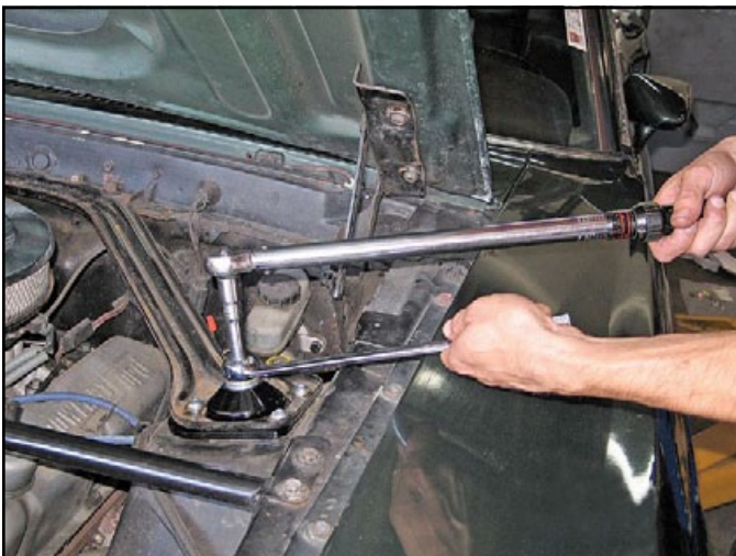
Under the hood, place a thick stem washer over the shock pivot stud, followed by an aircraft washer and half locknut, and securely tighten the upper-stud mounting hardware. The locknut is held with a wrench and the stem is turned counterclockwise using a 7/16-inch deep socket. Torque to 50 ft. lbs.
