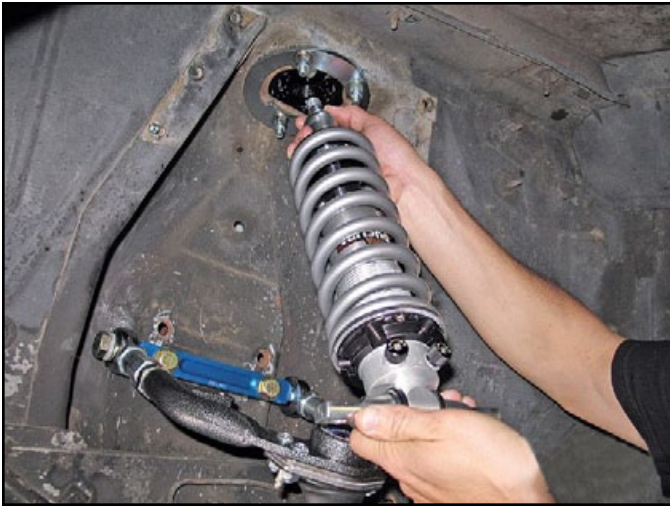
The assembled shock and spring can then be placed into the shock tower.
