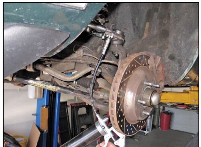
Be sure to lubricate any new parts, such as the ball joints in the new TCP upper arms.
