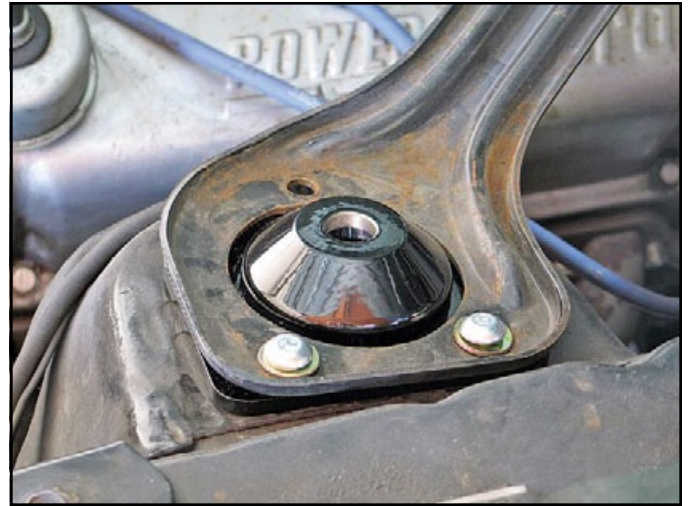
The shock-tower adapters drop into place under the hood with the radiused edge closest to the engine. We're showing it here in place with the export brace on top to illustrate the proper installation.
