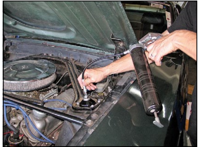
Install the supplied zerk fitting into the top of the shock stem and lubricate the pivot assembly with a grease gun.
