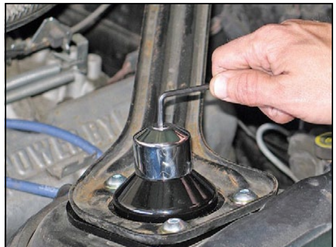
After lubrication, you can remove the zerk fitting to install the optional tower adapter caps. Place the tower adapter cap over the shock pivot stud and secure with the supplied flat-head cap screw. These polished stainless caps provide a clean completed look underhood.
