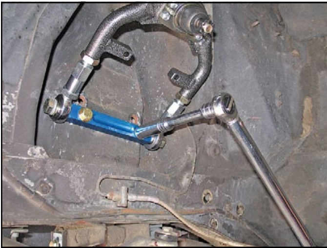
Drilling a set of new holes in the shock tower used to be required for installing new arms that have the correct suspension geometry built in. However that's no longer necessary as TCP offers a dropped pivot shaft that relocates the arms one-inch lower than the stock location. Our car already had the one-inch-lower holes so we went with standard TCP pivot shafts in the new arms. Once installed, the hardware is torqued to 95 ft. lbs.
