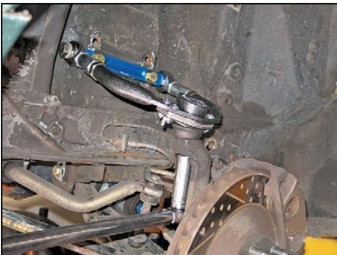
The new arm is then attached to the spindle and the castle nut is torqued to 75-80 ft. lbs. The new supplied cotter pin is then installed and the ends bent in opposite directions so they wrap around the stud.
