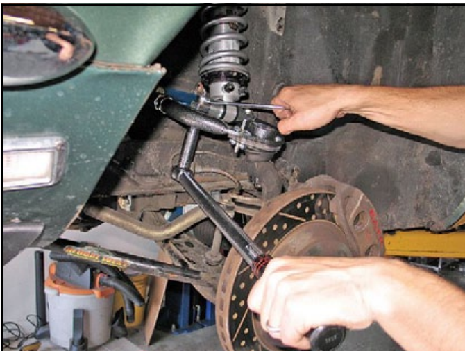
Bolt the shock's lower crossbar to the top of the upper control arm at the factory spring perch mounting location. Use the supplied hex bolts, flat washers, and locknuts, and torque them to 35 ft. lbs. A flat washer should be used under the bolt head and the locknut.
