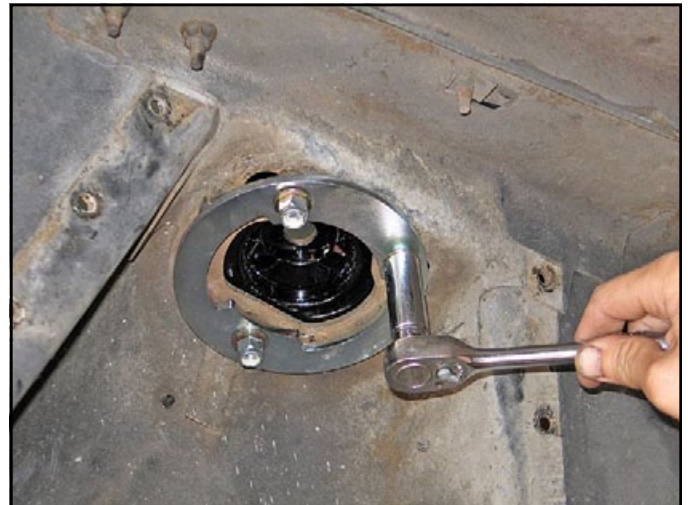
With the tower in place, install the backing plate underneath to sandwich the factory sheetmetal. Use the supplied three button-head bolts, flat washers, and locknuts to secure the mount and backing plate together as shown here. Now is also a good time to complete reinstallation of the export brace if your car has one.
