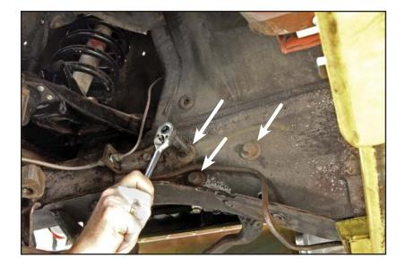
12. Remove the steering box from underneath the car. It may be necessary to remove the exhaust header or raise the engine to make room for the steering box to drop out.
