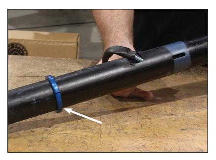
16. Insert the replacement steering shaft into the column tube.
