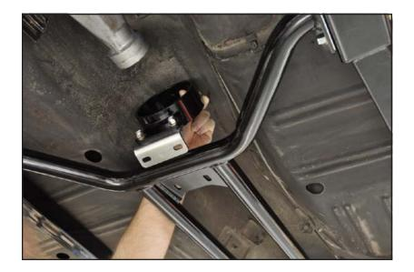
8. Loosely bolt the loop assembly to the center support using the 3/8-16 x 1" hex bolts, flat washers and locknuts
