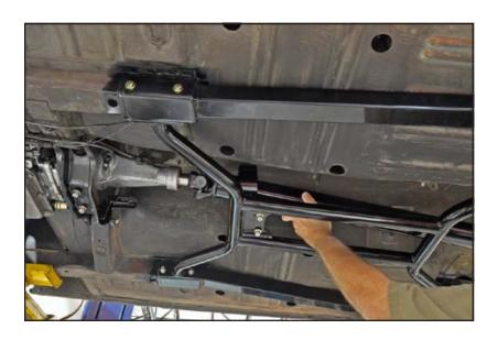
10. Install the rear u-bolts and hand tighten them only at this point.
