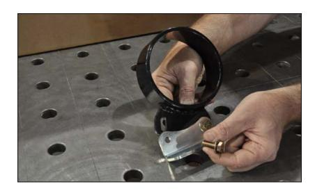
Slide a flat washer over the 3/8-16 x 1-1/4" hex bolt and insert it through the bracket and weldment. Place a second flat washer on the bolt followed by the locknut.
