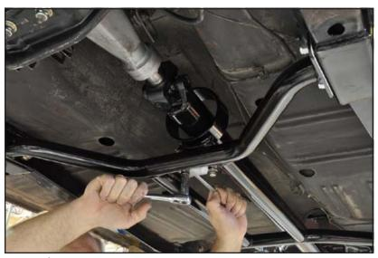
13. Center the loop around the driveshaft and tighten the bolts to 35 lb-ft.
