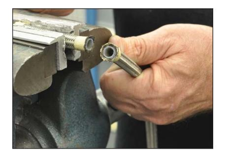
7. Disassemble the hose ends and slide the outer socket onto the hose with the threaded end of socket closest to the freshly cut end of the hose.
