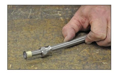
8. Place the brass ferrule in between the Teflon hose and steel braid as shown.
